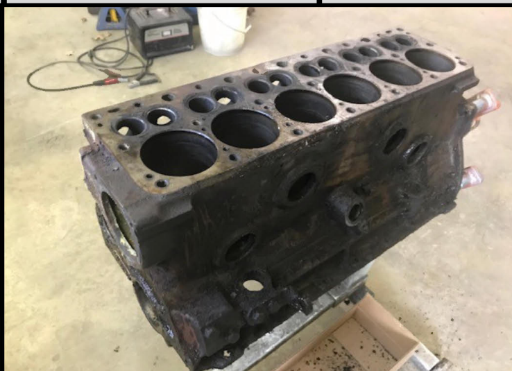
The (mostly) disassembled, grimy engine block.
