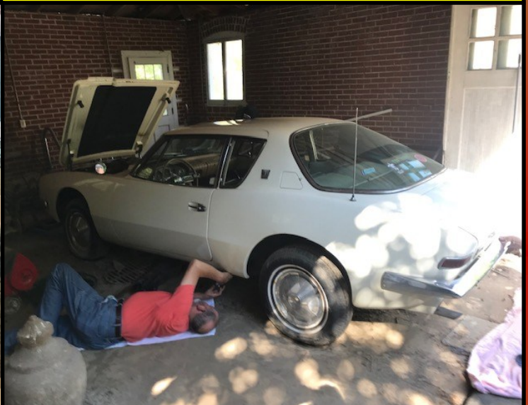
Gary taking a look at the undercarriage. "Hog troughs" and frame condition are important Avanti concerns.
