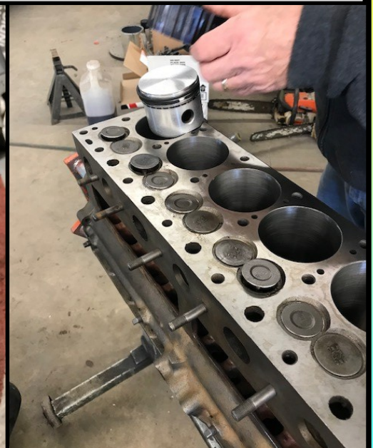
Installing crankshaft and main bearings.—A shiny, new piston with the rings installed.—Getting ready to install the new pistons.
