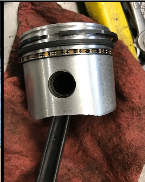
Installing crankshaft and main bearings.—A shiny, new piston with the rings installed.—Getting ready to install the new pistons.
