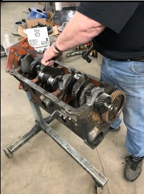
Installing crankshaft and main bearings.—A shiny, new piston with the rings installed.—Getting ready to install the new pistons.
