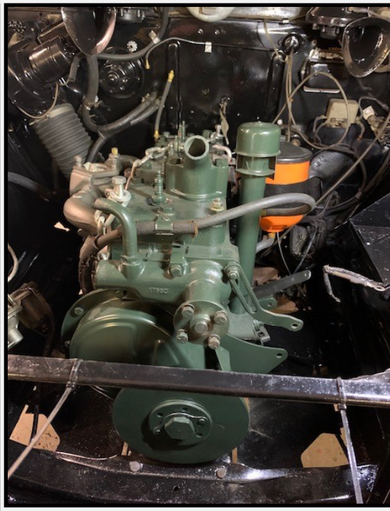
The rebuilt engine just nestled into the freshly painted engine bay. Looking pretty good!
