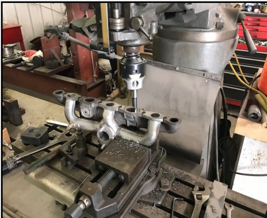
Milling the "block face" of the manifold for a better seal. The exhaust port openings were pitted from the heat and there was also some warpage.
