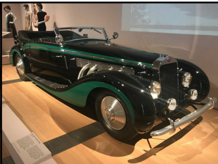
A sleek, 1937/38 Delage featuring a special, lowered frame and a 4.7L straight-8 engine backed by an electronically motivated 4-speed transmission.
