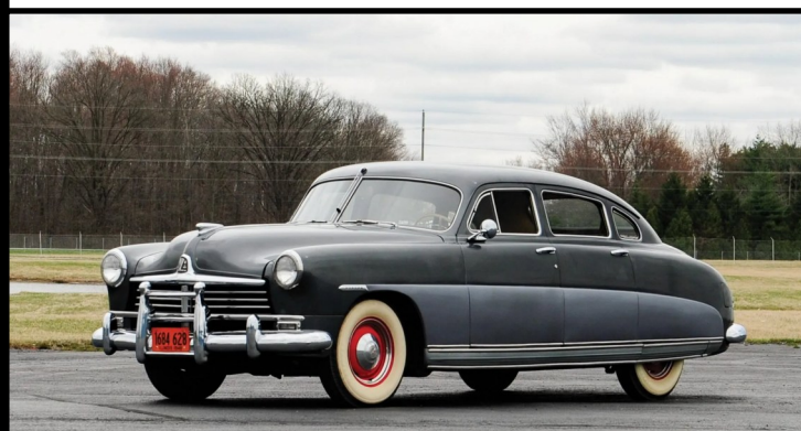
Introduced in 1948, Hudson's dramatic "step down" design was not only modern looking but also delivered good handling and a smooth ride.
